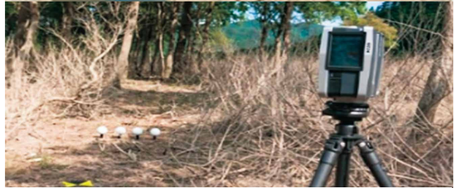
[Figure 3] Measurement of submerged forest by drone and ground laser
